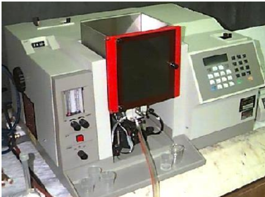
Fig 1: Picture of a flame atomic-absorption spectrophotometer apparatus (13)
